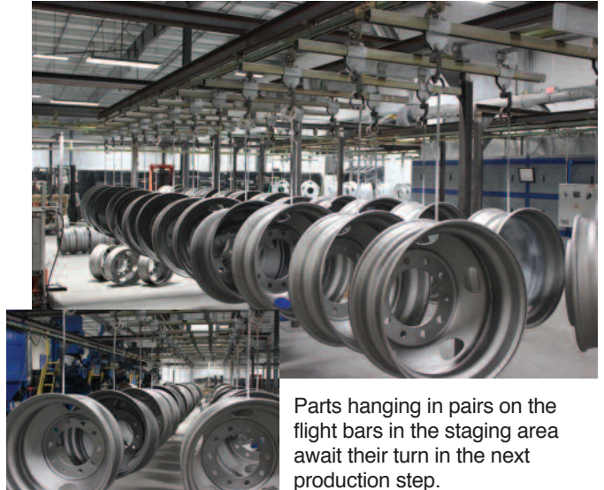
Parts after exiting the primer booth and before entering the catalytic IR primer gel oven.
