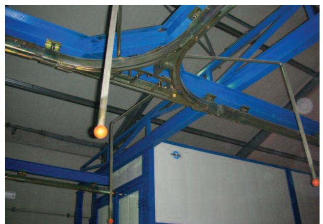
Triple tongue switch used to transfer flight bars.
