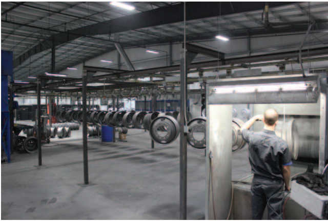
Primer application booth is shown with one of the staging areas seen in the background.
